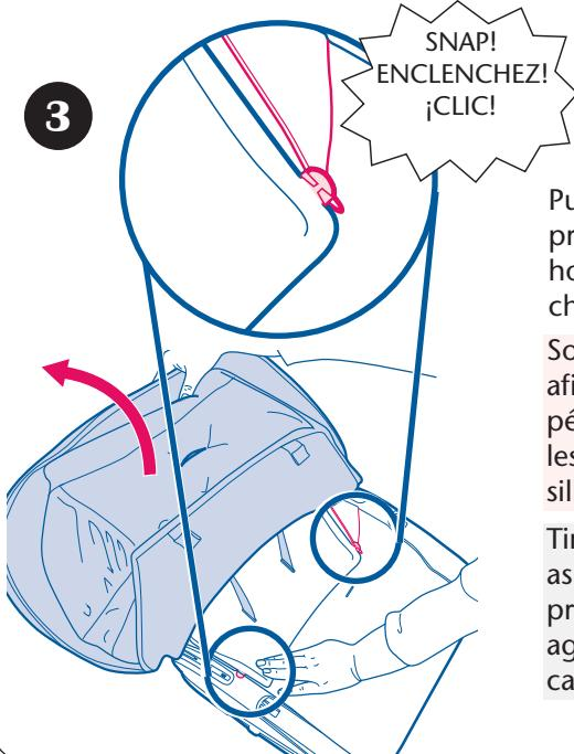
Pull seat pad up in order to press the pegs into the holes at the bottom of the channel.
